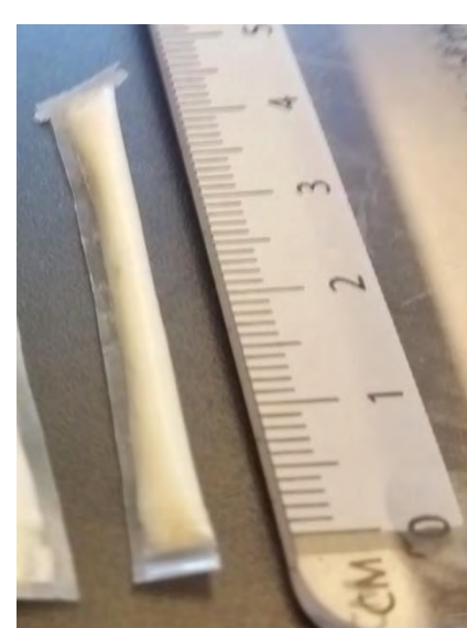
Full-scale TAF-TFPD prototype devices 4 cm long x 2-2.5mm diameter
